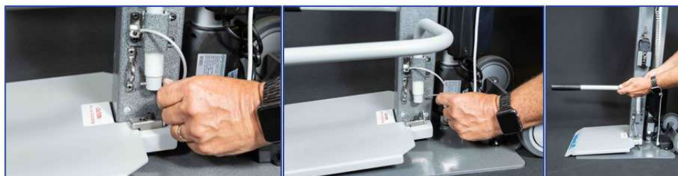
Remove Locking Pin Then Lift Handle Upward
